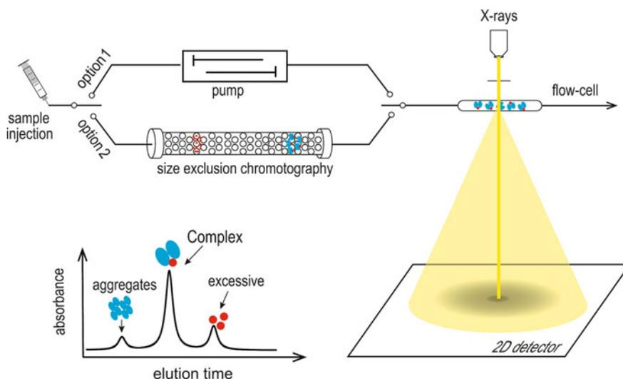
**Fig. 14.4** Experimental SAXS data acquisition. Two setups are routinely used: one with a simple flow-cell (*top*) and the other coupled with online chromatography (*bottom*) (Modified with with permission Yang 2014)
